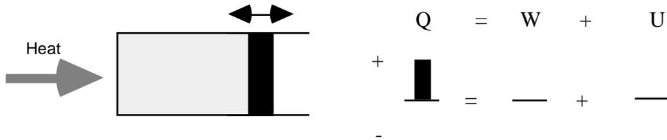
Container is completely insulated, piston is free to move and the external pressure is reduced.
