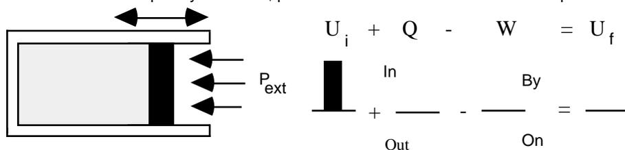
The container is immersed in a very large container of water at a temperature T. The piston is pushed in a distance "d."
