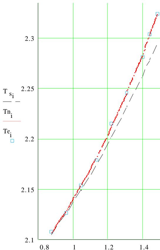
Fig. 3. Experimental Data  $T_e$  vs.the initial angle. The numerical integral evaluation  $T_n$  and the evaluation by the elliptical integral series representation  $T_s$  are also plotted for comparison.
